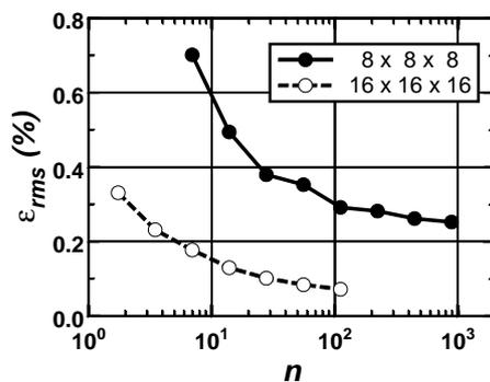
Fig. 3. Difference  $\varepsilon_{\text{rms}}$  between the particle sum (1) and the pixel sum (3) as a function of number  $n = N_p/N$  of particles per pixel, at two fixed pixel discretizations. The two velocities are computed at the centers of all pixels, and  $\varepsilon_{\text{rms}}$  is the root-mean-square discrepancy, normalized as a percentage of the maximum velocity norm.
