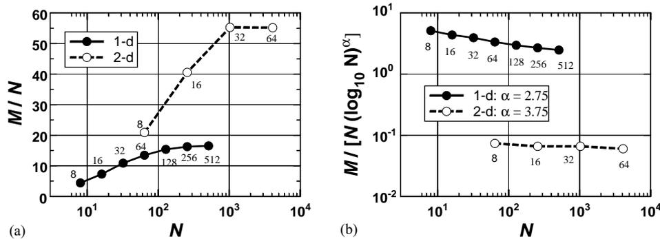
Fig. 6. Scaling of the operation count  $M$  with the number of pixels  $N$  for wavelet compression of the 1D and 2D kernels defined by Eqs. (10) and (11). Numbers by the points indicate the linear pixel resolution. (a) Fixed accuracy  $\epsilon_{\max} = 1\%$ ; (b) increasing accuracy  $\epsilon_{\max} \propto N^{-1/2}$ .
