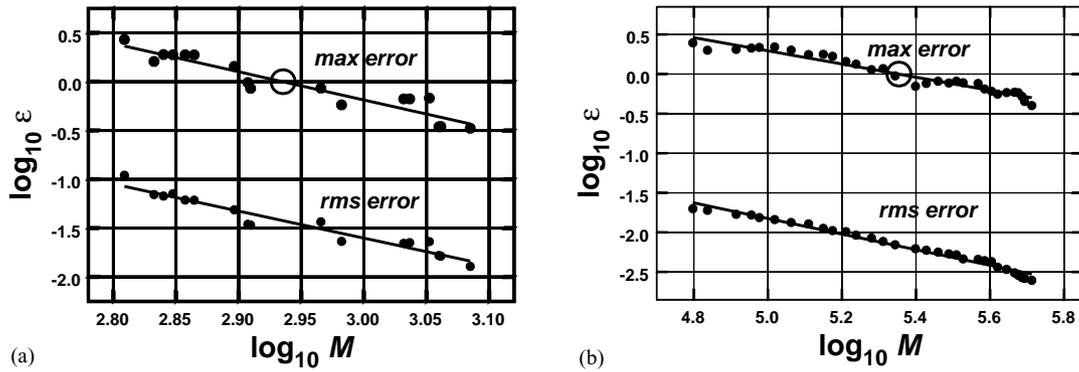
Fig. 5. Error  $\epsilon$  in the output signals  $\psi_i^{(1)}$  and  $\psi_{ij}^{(2)}$  as a function of the number  $M$  of retained wavelet coefficients in the truncated kernel arrays  $\tilde{K}_{il}^{(1)}$  and  $\tilde{K}_{ij,lm}^{(2)}$  at fixed, 16 pixel resolution. (a) 1D; (b) 2D.
