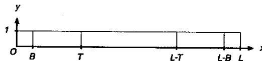
Fig. 4. Domain of solution, consisting of one of the two flow channels in Fig. 3. The entrance and exit regions are given by 0 < x < T and L - T < x < L , respectively. Flow occurs through the porous sections 0 < x < B , L - B < x < L of the upper wall. The flow fields at the ends are matched to a fully developed parabolic velocity profile in the middle section, along x = T and x = L - T , for which T = B + 3 was found to be sufficiently large to encompass the entire flow rearrangement without introducing any significant inaccuracies in the matching.
